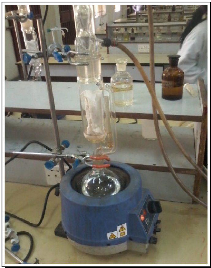
Figure 1. Soxhlet extraction in progress
