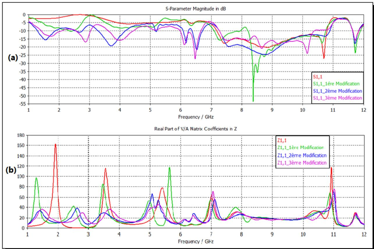
**Figure 2.** (a) Return loss, (b) Real part of the input impedance
