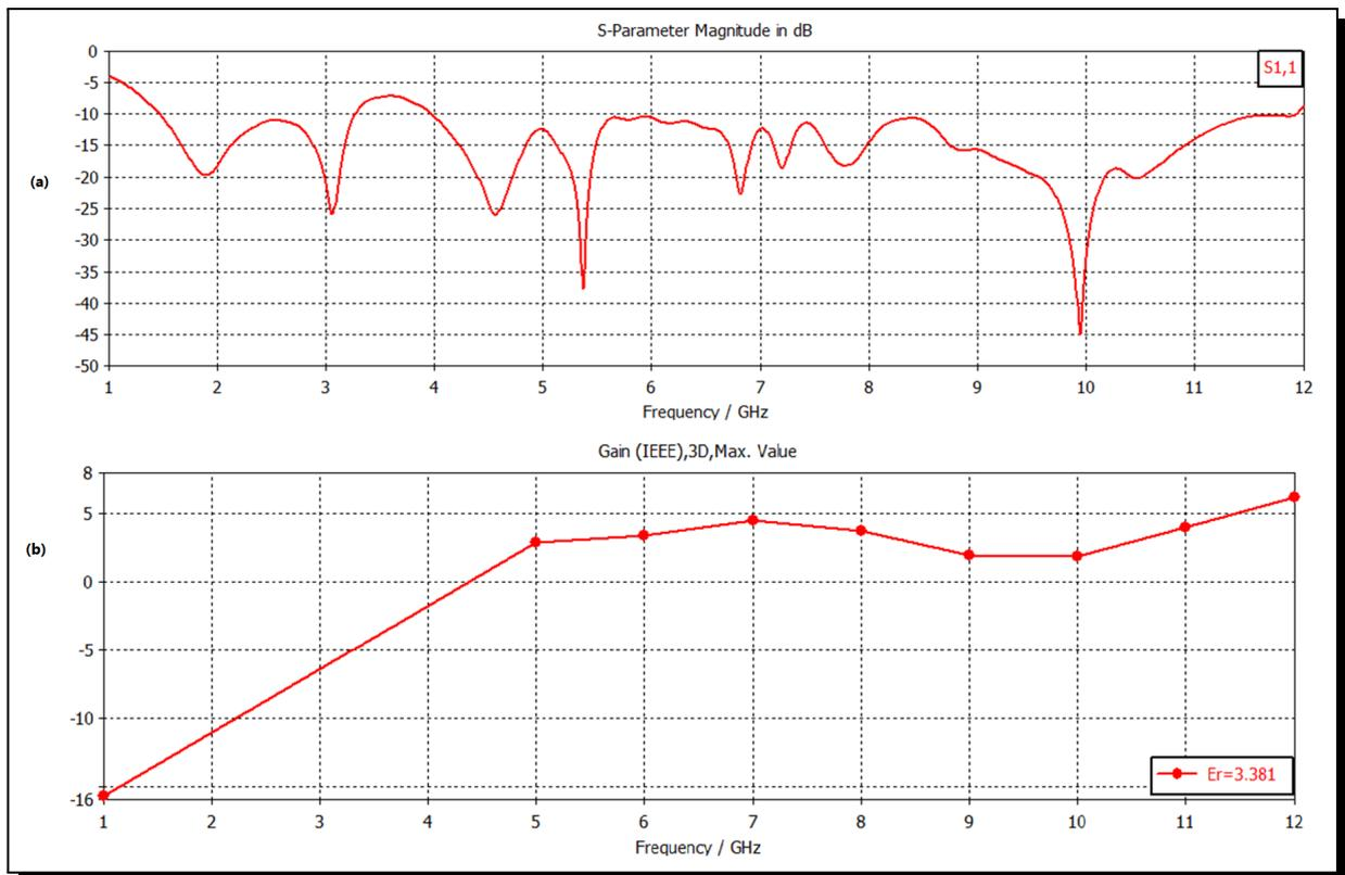
Figure 7. Return loss, Final antenna gain
