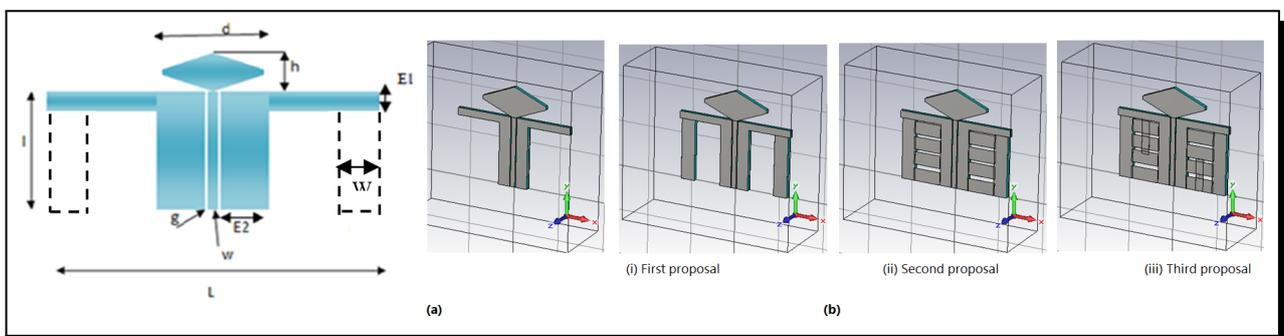
Figure 1. (a) Geometry of the initial diamond monopoly antenna, (b) Geometry of the proposed antennas
