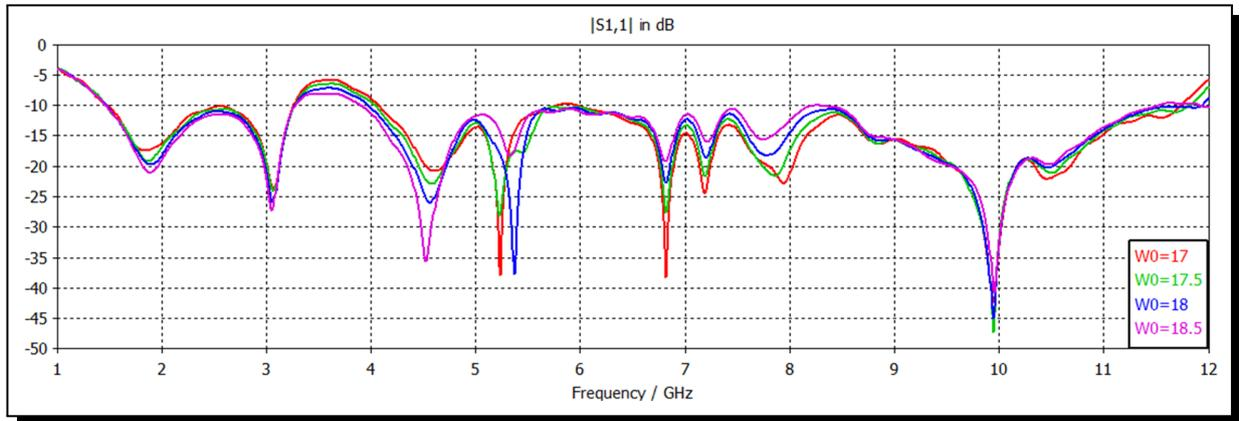
Figure 6. Return loss variation according to the parameter  $W_0$
