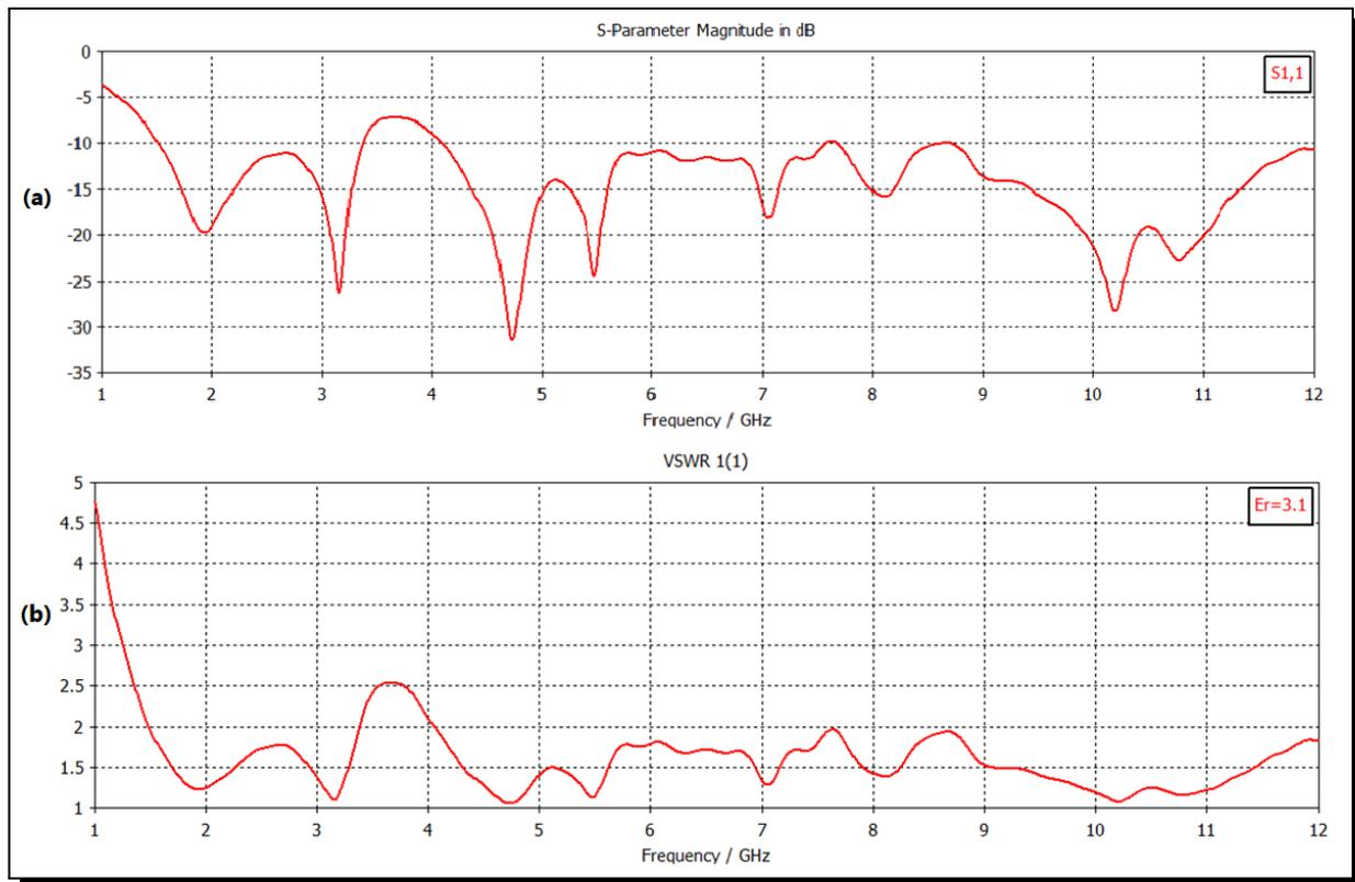
Figure 5. Return loss, Stationary wave ratio
