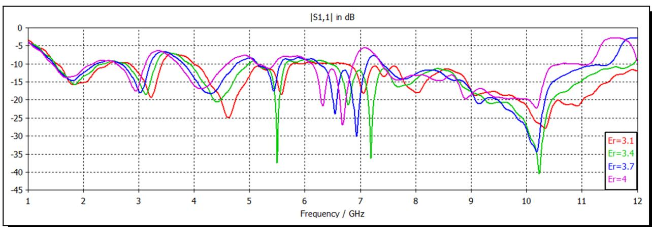
**Figure 3.** Variation of the return loss according to the parameter  $\epsilon_r$ .
