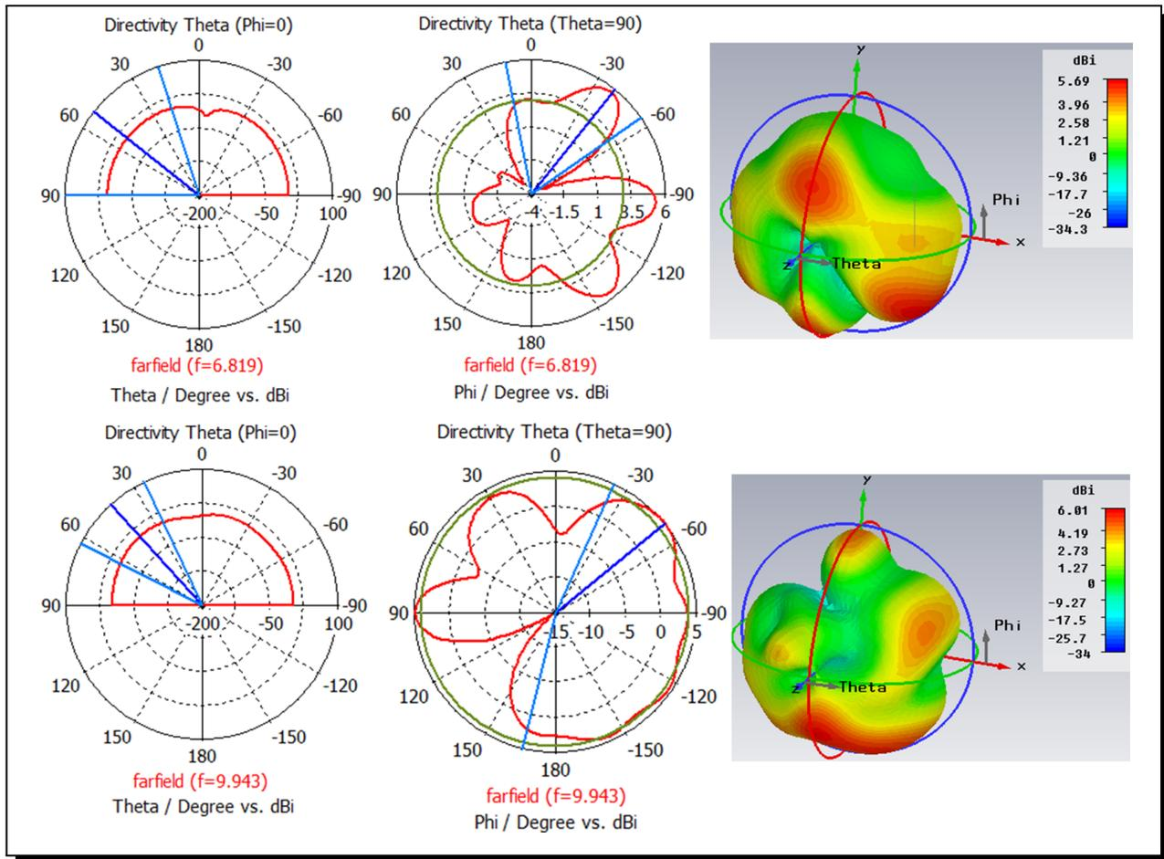
**Figure 8.** Radiation diagrams in 2D and 3D at the different frequencies
