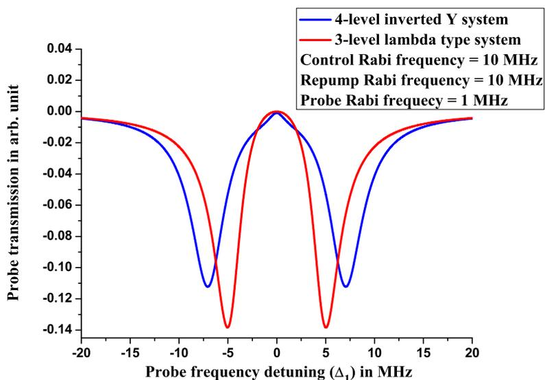
**Figure 5.** (Colour online) Plot of probe transmission vs. probe frequency detuning under Doppler free condition for a four-level inverted Y-type system and a three-level  $\lambda$  type system for a fixed set of Rabi frequencies of the control, probe and repump fields (mentioned in the graph).
