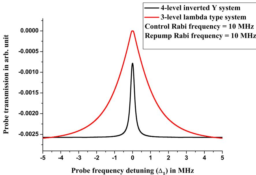
**Figure 4.** (Colour online) Plot of probe transmission vs. probe frequency detuning for a four-level inverted Y type system and a three-level  $\Lambda$  type system. The values of the control, probe and repump Rabi frequencies have been kept fixed at 10 MHz, 1 MHz and 10 MHz respectively during the simulation.
