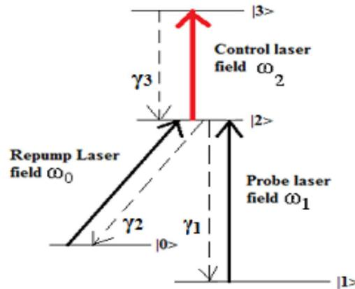
**Figure 1.** (Colour online) Inverted Y type level scheme.
