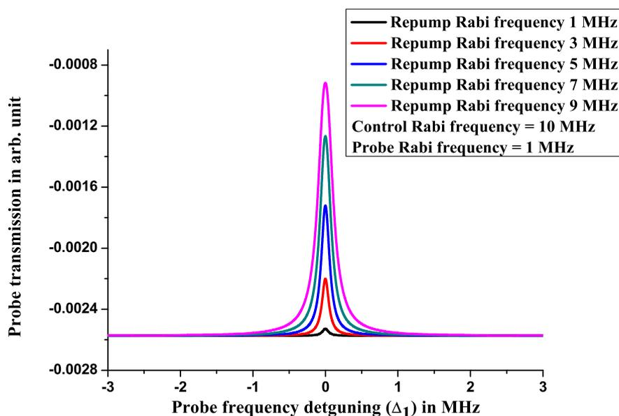
**Figure 3.** (Colour online) Plot of probe transmission vs. probe frequency detuning at different values of the repump Rabi frequency ( $\Omega_0$ ) under Doppler broadened regime. The probe Rabi frequency ( $\Omega_1$ ) and the control Rabi frequency ( $\Omega_2$ ) are held fixed at 1MHz and 10 MHz respectively during the simulation. The complete Doppler background is missing here since we have shown the zoomed part around zero probe detuning.
