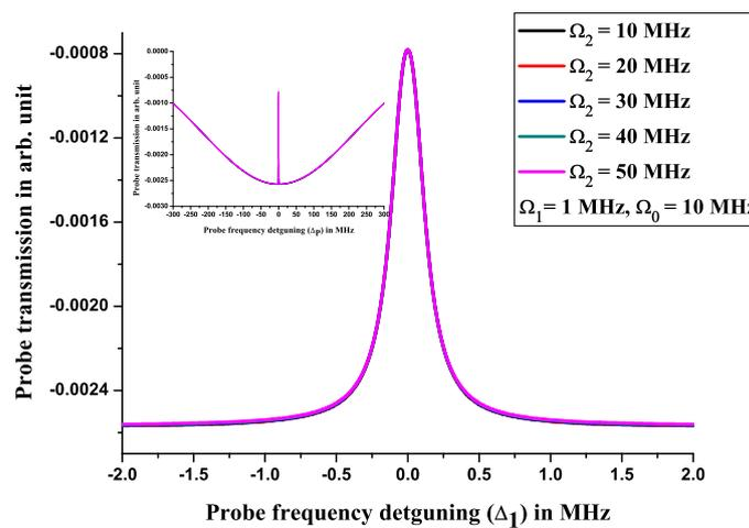
**Figure 2.** (Colour online) Plot of probe transmission vs. probe frequency detuning at different values of control Rabi frequency ( $\Omega_2$ ). Probe Rabi frequency ( $\Omega_1$ ) and repump Rabi frequency ( $\Omega_0$ ) are held fixed at 1MHz and 10 MHz respectively during the simulation.
